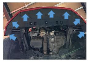
You will now need to unclip and unbolt both sides of the top of the front bumper. Use a 10mm socket to remove the bolts and apply pressure using a flat-bladed screwdriver to release the clips. Also pull the rubber edge away which goes from one side of the engine bay to the other.
