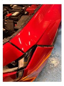
6. Unclip all pf the wiring connections from the front bumper, you will also need to release the washer bottle hose so make sure to have something in place to catch the excess fluid.
