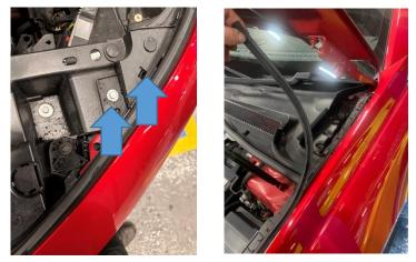
3. Remove the 10mm bolt hidden under the trim which is securing the bumper to the wing on top of the headlights.
