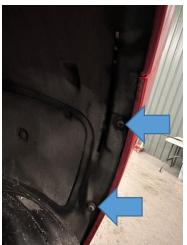
5. You can now pull the edge of the front bumper to release it from the wings, but do not fully remove the front bumper yet.
