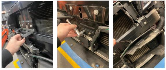
8. Remove the two 10mm bolts from the bracket to the crash bar and then remove the four T27 Torx bolts securing the plastic air scoop. You do not need to reinstall these parts.
