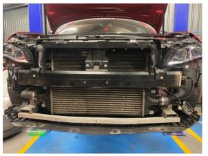
Remove the intercooler by releasing the two 10mm bolts either side that secure it in place. Then loosen the spring clips securing the boost pipes using a trim removal tool by lifting them until you hear they click. The intercooler can then be tilted towards you and lifted out.
