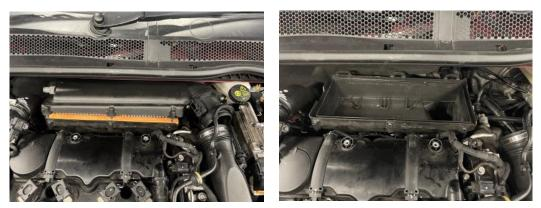
5. Now remove the other T15 Torx bolt from the MAF housing in order to separate it from the air box lid, as shown. You can also remove the O-ring as you will not be using it.
