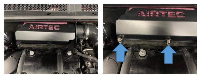
11. Finally, reinstall the engine cover and check that everything has been secured correctly.
