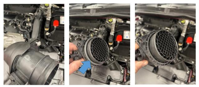
6. Using the supplied hardware, install the bracket onto the MAF housing with two M6 bolts, nuts and washers either side, as shown. Secure using a 5mm Allen key and 10mm spanner.
