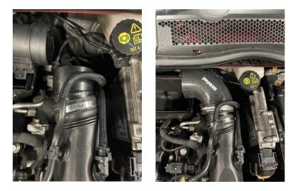
8. You can now install the bracket with the MAF sensor housing by reusing the engine cover stud removed in Step 2 and installing the housing into the Pro Hoses silicone connector with the supplied jubilee clips. Then plug the MAF sensor wiring back in, install the AIRTEC air filter into the air box and secure using a hose driver.
