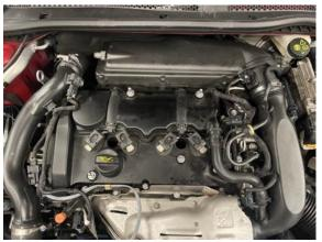
2. Remove the two engine cover locating studs using a 10mm spanner and then loosen the three T15 Torx bolts securing the air box lid in place.
