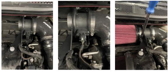
9. Reinstall the other engine cover stud removed in Step 2 with the supplied spacer, as shown.
