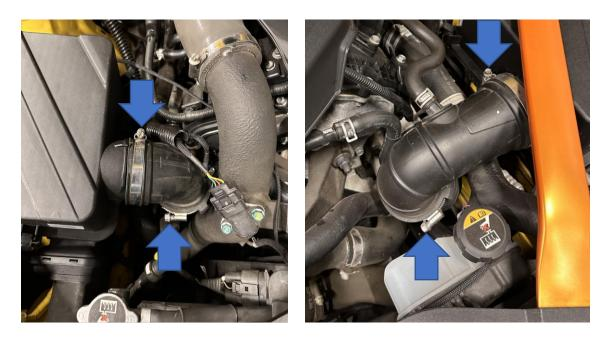
2. Using hose clamp pliers, remove the three hoses that are attached to the right-hand side intake. It is easier to disconnect the larger hose from the car side, at the front of the engine, as shown. On the left-hand intake there is just one hose to unclip from the front of the engine, as shown.
