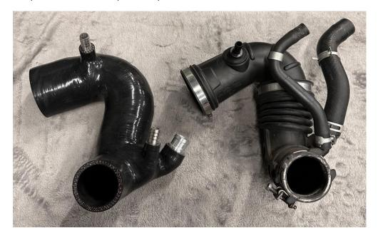
4. Install your new Pro Hoses intakes using the supplied jubilee clips in reverse of Steps 1 to 2. Make sure you reconnect all the ancillary hoses using the provided jubilee clips for each hose.
