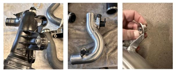
11. On the right-hand boost pipe, undo the T27 bolt holding the pipe to the gearbox and then you will need to remove the pipe from above. Take care when removing as the wiring and coolant lines run in close proximity.
