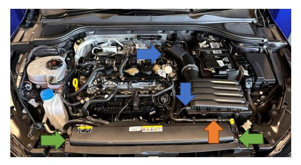
2. Remove the recirculation hose from the car by using a pair of hose clamp pliers to squeeze the spring clip and then pull around the base of the hose to remove it. Then release from the two trim clips holding it onto the boost pipe.
