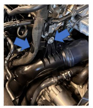
4. Undo both jubilee clips holding the hose onto the turbo and then remove from the car.
