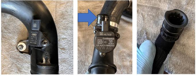
10. The rubber bushings and bolts can now be removed from the original by using a trim tool or similar to get under the head of the washer and pulling it up. Repeat this process for both bolts and then install the supplied spacers with bolts as shown. The new cold side pipe can then be refitted and reconnected in reverse of removal.
