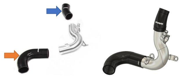
13. For the right-hand boost pipe, locate the three silicone hoses below from the kit and install the highlighted with the blue arrow onto the turbo along with the short aluminium hard pipe, as shown below. Then add the silicone coupler highlighted with the orange arrow with the jubilee clips attached, but not tightened at this stage.
