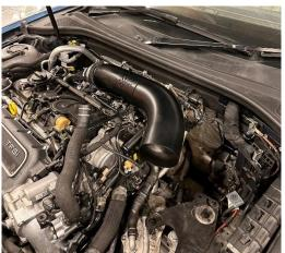
11. Clip the vacuum hose back onto the new pipe and reinstall the hose and tension clip removed in Step 2. If necessary, loosen the clip on the other end of the hose and rotate it to allow additional clearance.
