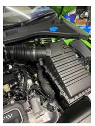
5. Two of the original rubber mounts are used to install your new AIRTEC Motorsport heat shield, so remove them from either the air box or check if they remained in the car.
