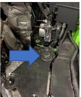
6. On the intake pipe, remove the vacuum pipe by squeezing the clip and pulling it. Then locate the bolt hidden from view on the underside of the pipe and remove with a T27 Torx bit.
