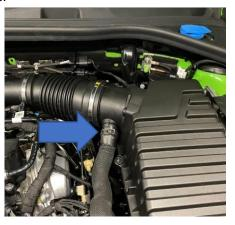
3. Use a trim clip removal tool or similar to unclip the breather hose from the air box by pulling it towards the front of the car. Once removed, slide the metal clip up and off the air box.
