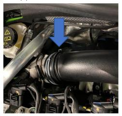
8. Install the new silicone reducer onto the turbo elbow using the 100mm jubilee clip supplied.
