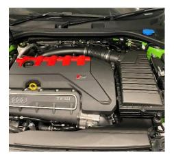
2. Using hose clamp pliers, release the tension clip from the hose secured to the air box and then disconnect the hose.
