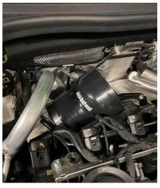
9. Install the bracket onto the car as pictured below by first installing the supplied M6x25mm Hex Head bolt with washer through the **back** of the original bracket until tight and then install the bracket onto the bolt and secure using an M6 nut and washer.
