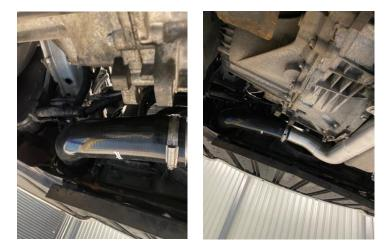
6. To install the cold side pipes, start by locating and removing the hose to the throttle body from the top of the engine bay. Then fit the straight silicone hose onto the new cold side pipework as shown and fully tighten with a supplied jubilee clip. Attach to the throttle body and once happy with the fitment, tighten the jubilee clip from the top of the engine bay.
