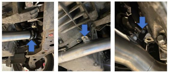
5. Install the final silicone hose for the hot side in place by fitting it onto the alloy pipework and directly to the intercooler as shown. Use the supplied jubilee clips and fully tighten.
