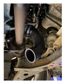
3. You will now need to install the mounting bracket supplied onto the new hot side boost pipe as shown. Use a 13mm socket to secure the supplied Hex Head bolt with washer in place, but do not fully tighten yet as you will need some adjustment later.
