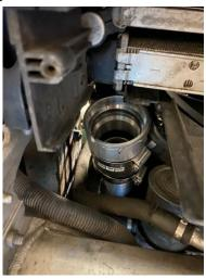
5. Finally, refit the intercooler and connect the boost pipe reusing the original spring clip. Once happy with the fitment, fully tighten the jubilee clips and make sure everything is tight and secure. Then refit the cold side boost pipe and the undertray as removed in Step 1.
