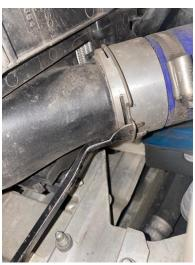
2. Follow the left-hand side/hot side boost pipe up to the turbo and release the spring clip that attaches it. You can then remove the pipe from the engine bay.
