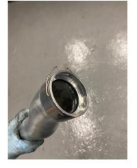
4. Install the first part of new hot side pipework onto the turbo reusing the original spring clip. With that in place, fit the silicone reducer and then the billet connector, as shown. Leave the jubilee clips lose to allow movement to align it.
