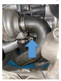
3. Swap the O-rings and spring clips over from your original pipework onto the new
