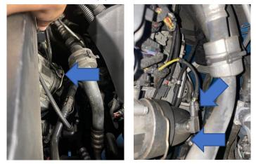
3. Remove the sensor from your original pipework and install it into the new one using the provided fixings. You will also need to swap over all the O-rings and clips from your original pipework, as shown.
