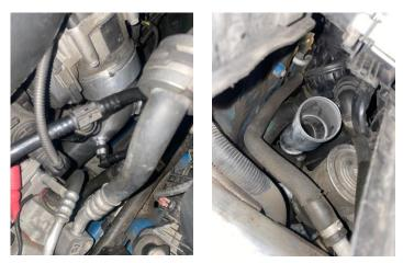
5. Finally, refit the intercooler and connect the boost pipe reusing the original spring clip. Once happy with the fitment, fully tighten the jubilee clips and make sure everything is tight and secure. Then refit the hot side boost pipe and the undertray as removed in Step 1.
