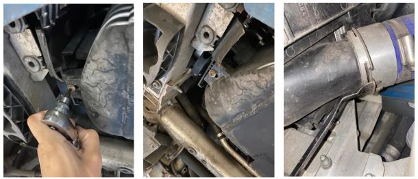
2. Follow the right-hand side/cold side boost pipe up into the engine bay and release the spring clip attached the throttle body. Then unplug the sensor that is attached to it, unclip the vacuum hose and remove the pipework from the car.
