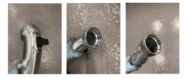
4. Install the first part of new cold side pipework onto the throttle body reusing the original spring clip and plug the sensor back in along with the vacuum hose. With that in place, work down by fitting the silicone reducer and then the second pipe. Leave the jubilee clips lose to allow movement to align it.
