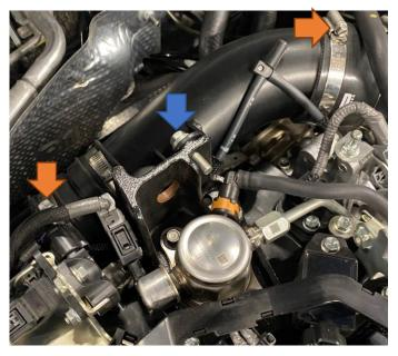
7. Remove the breather and vacuum hoses from the original pipe. You will need to unclip the other vacuum lines routed along the original pipe.
