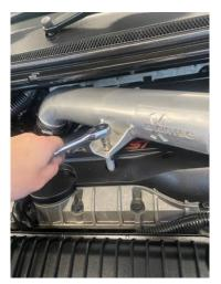
9. Remove the MAF sensor from the original intake pipe, install into the new crossover pipework and plug in the MAF sensor wiring extension loom as shown.
