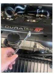
8. Install the crossover pipe into the original hose and secure. Then install the bracket onto the pipework and attach to the thread located on the back of the engine. Also fit the crossover onto the threaded boss as shown and secure.
