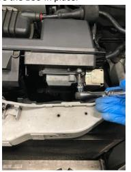
5. Unplug the MAF sensor then remove the vacuum pipework by releasing two T15 Torx bolts. You can then remove it from the plenum by holding the red part and pulling the pipe.
