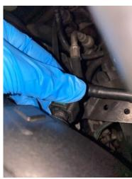
3. Remove the slam panel by using a screwdriver and a trim tool to remove all eight plastic push clips. Once removed, you will be able to access the air feed, which will also need to be removed by releasing the two push clips.
