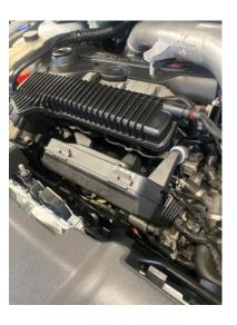
12. Finally, install the air filter and trumpet with the supplied jubilee clips. **Do not over tighten – the trumpet as it can crush.**
