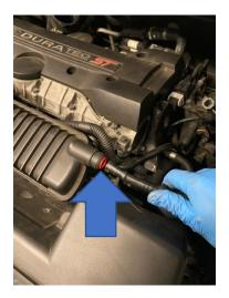
6. Disconnect the brown plug attached to the vacuum pipework and then release the ECU by turning it onto its side and carefully placing it down in the engine bay – there is no need to unplug it. The air box can now be removed by pulling it from its rubber mounts.
