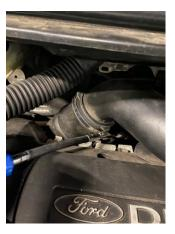
2. Now remove the two bolts that are located behind the crossover pipe. You will also need to remove the vacuum pipe from the crossover by pressing on the green tab and pulling the pipe off. The crossover pipe can now be removed from the car.
