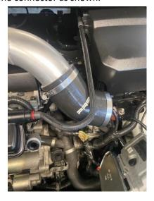
11. Now install the AIRTEC Motorsport ECU holder. Carefully turn the ECU to the correct position as shown then align it with the back of the casing. Remount the ECU into the holder by reusing the Torx bolts removed in Step 4. You can then clip the front of the casing on and push the fittings on the back of the casing through the tabs that located the original air box.
