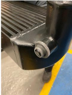
14. You can now install the AIRTEC Motorsport intercooler by using the provided M8x20mm bolts to mount the intercooler to the crash bar brackets, two each side. You will also need to reuse the original bolt removed in Step 11 for the lower right-hand side bracket.
