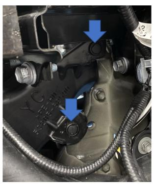
9. Remove the crash bar by undoing the 10mm nut and four 14mm bolts each side. The crash bar will then pull away.
