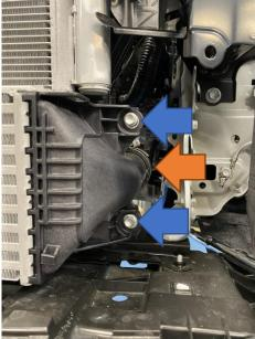
12. Remove the undertray by removing four 10mm bolts from the tabs on the back of the undertray.
