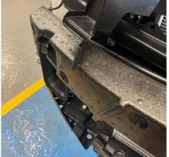
7. Remove the lower plastic trim by removing the three plastic clips using a trim removal tool.
