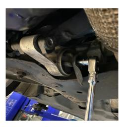
3. The stock torque mount can now be removed.
