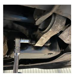
2. Now remove the 17mm bolt securing the other end of the torque mount in place.
