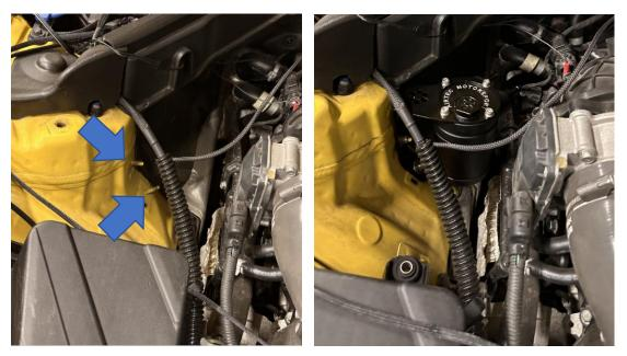
4. Finally, install the supplied hoses with jubilee clips together with the hose separator in the location as pictured. Make sure everything is tight and aligned correctly.
