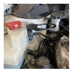
5. Attach the AIRTEC Motorsport catch can to the bracket using the supplied M5x12mm Button Head bolts and washers.
