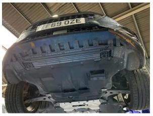
2. Now remove two T27 bolts from either side of the wheel arch liners.
