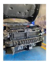
8. Remove the two 10mm bolts from the top of the crash bar.
