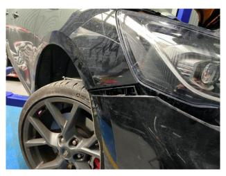
6. Now unclip the wiring harness from inside the driver's side (right-hand drive car) arch liner and unclip two harness clips.
