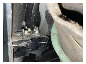
5. Release the bumper from the wing brackets by carefully but firmly pulling from the car.
