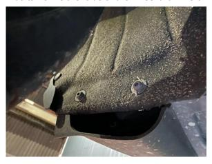
3. Remove the six 10mm bolts along the top of the bumper, as well as the two trim clips and two T27 Torx bolts.
