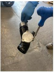
5. Remove the O-ring from the original pipework and install it into the new AIRTEC Motorsport pipe. Then swap the clip over, making sure it's fitted exactly as shown below. You will also need to swap the clip that secures the wiring loom over as well.
