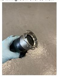
6. Install the charge pipe by attaching it using the same clip and reattach the wiring loom. Then install the silicone pipe onto it using the supplied jubilee clips.
