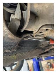
2. Locate the boost pipe coming from the turbo at the back of the engine. Release the wiring from the clip attached to the pipework then release the clip securing the pipework to the turbo. Release it by lifting the clip up with a flat-bladed screwdriver until the clip makes a 'click' sound.
