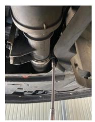
4. If you are **not** installing a recirculation valve, you can install the supplied O-ring onto the recirculation valve blank and fit to the pipework using a 5mm Allen key.
