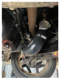
7. The pipework can now be installed into the silicone hose and mounted onto the car by reusing the original 10mm bolt removed in Step 3. Then complete the installation by attaching the pipe to the original boost hose using the original jubilee clip.
