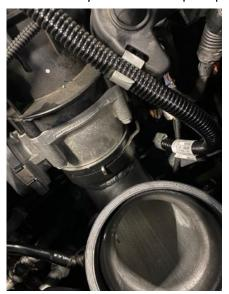
8. Finally, you can reinstall the pipe removed in Step 5 and install the silicone hose with provided jubilee clips in place. Then reassemble the car in reverse of Steps 1 to 4, making sure that everything has been secured correctly in place. When everything has been refitted check the chargecooler coolant level and top up/and bleed the system if required.
