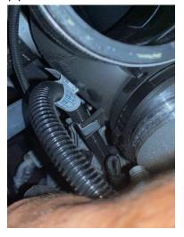
6. Now remove the original charge pipe by lifting the exposed tab that secures it to the engine. Pull the tab all of the way out and remove the pipe.
