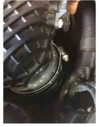
5. Now locate the original J-pipe from the throttle body. You will need to apply pressure to the clip securing the vacuum line to the original pipework to remove. Then unclip the wiring from the pipework as well.
