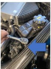
3. Unplug the sensor from the back of the chargecooler (orange arrow)). Then release the spring clips securing the coolant lines at the front. Clamp both hoses to stop fluid leaking and also have something on-hand to catch any excess that will spill before removing the lines.
