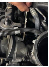
7. The new J-Pipe can now be fitted in place. Make sure that you have installed the supplied O-ring and spring clip to be able to fully secure the J-Pipe in place.
