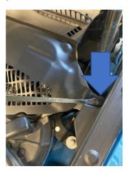
2. You will now be able to access the six 13mm bolts securing the strut brace in place. You will also need to remove the 10mm bolt securing the coolant bottle to the brace.
