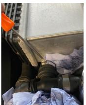
4. Loosen both jubilee clips on the left-hand side of the chargecooler as well as the jubilee clip on the lower right-hand side. Once they have been loosened, you can lift the chargecooler up from the rubber mount and remove from the engine bay.
