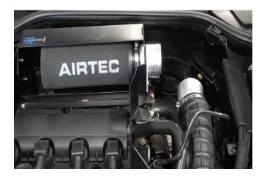
5. Install the air guide blank on the left hand-side of the airbox using the supplied M6 fittings then on the right-hand side secure the filter adapter onto the side of the air box using the supplied M6 fittings. You can now also install the silicone pipework from the alloy pipe connector to the filter adapter.
