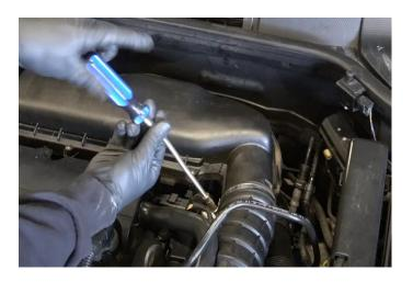
2. Now remove the x4 T20 torx screws from the lid of the airbox and remove the lid and stock air filter.
