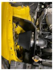
6. Install the right-hand side of the intake by placing the heat shield in first and aligning the mounting tabs with the exposed threads in the engine bay. Once you have located the two fixing points, secure them in place using the other two supplied M6 bolts and washers. Now install the filter as per the left-hand side and tighten.
