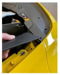
2. Remove the strut braces from the engine bay by undoing the four 13mm bolts securing them in place. Once they have been removed, you will be able to release the jubilee clips to the air boxes and then remove them from the car.
