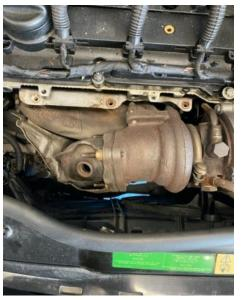
2 Remove the three 13mm nuts securing the downpipe to the turbo. You will also need to remove the three studs (highlighted with blue arrows), which you can do by tightening two nuts together on each stud and using the nut closest to the downpipe to unwind the stud.
