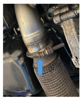
Install your new AIRTEC Motorsport downpipe from the top of the engine bay.
