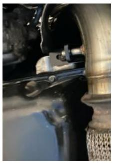
8 Finally re-install the lambda sensors and heat shield in reverse of Steps 1 and 3. Then check everything has been tightened correctly.
