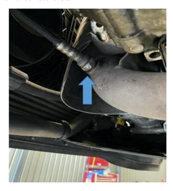
4 Now remove the two 13mm nuts (highlighted with blue arrows) securing each side of the original mounting bracket in place.
