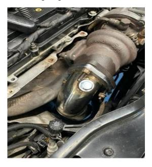
7 Re-install the exhaust clamp removed in Step 5 and then install the AIRTEC Motorsport mounting bracket using the 13mm nut removed in Step 4
