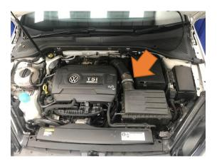
2. Now remove the vacuum pipe from the original air box.
