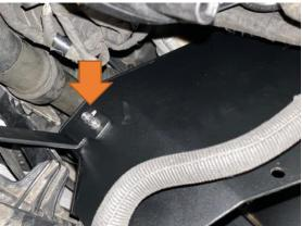
7. The air filter can now be installed by securing it to the intake pipe using the jubilee clip supplied. Also reattach the vacuum line removed in Step 2 to the new pipe.
