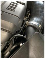
8. Install the enclosed air box lid by placing it on top of the base and align the tabs with the allocated holes. You can now secure the lid using the supplied push fittings. Finally, check everything is aligned, tight and secure.
