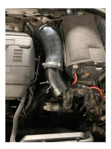
5. Now install the base of the new air box by securing it to the bracket on the intake pipe with the supplied M6x16mm bolt and washer, as shown. Then place the alloy spacer underneath the back of the air box base where the original air box was originally mounted, as shown. You can then secure it in place using the supplied M6x70mm bolt and washer with a 5mm Allen key.
