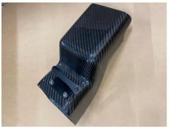
3. Locate the hole in the slam panel as shown and align the bracket to it. Then secure in place using the provided M6 bolt with a nyloc nut and washers.
