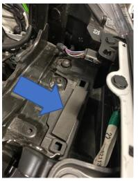
2. Now attach the bracket onto the air feed using the two M6 bolts with four washers and two nyloc nuts supplied. Make sure that the bracket is secured the correct way, as shown.
