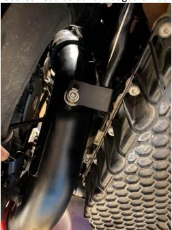
11. Install the silicone hose onto the turbo and secure using the provided jubilee clip. Once secured, you can install the hot side pipework into the silicone hose.
