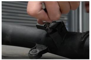
8. Install the silicone hose onto the throttle body and secure the jubilee clip using a
