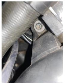
3. Loosen the jubilee clip from where the stock hose meets the throttle body. Once loose this can be pulled down and out from underneath the car.
