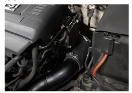
12. Now the hot side pipework is roughly in place you can install the silicone hose which goes from the alloy pipework to the intercooler.
