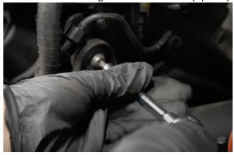
5. You will now need to loosen the jubilee clip from the hot side boost pipe that connects to the turbo. Once loose, it can be removed from the car.
