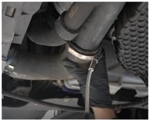
2. Remove the cold side pipe work by loosening the two T27 Torx bolts securing it in place. You will also need to unplug the sensor, which is located on the pipework.
