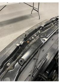
5. The air duct can now be removed from the car by releasing the plastic tabs attaching it to the crash bar.
