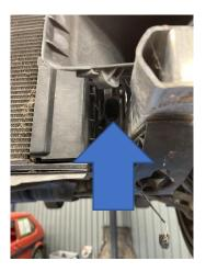
10. Drain the coolant from your original radiator and hoses by releasing the hose clip from the lower offside of the vehicle. Make sure to have something in place to catch the excess fluid.
