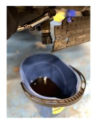
11. You can now fully remove the original radiator by releasing the hose on top of the radiator.
