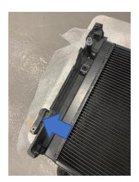
13. You can now install the radiator onto the car in reverse of removal, making sure to slot the pin into the rad pack. Then secure the radiator in place by reusing the T27 bolts that you previously removed in Step 9.
