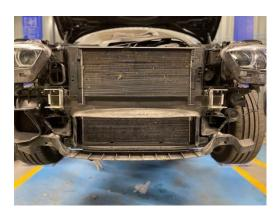
7. You will now need to remove both of the brake cooling guides by removing the trim clips with a trim removal tool on both sides of the guide. Then you can remove the lower air feed for the radiator and remove the two E11 bolts from the lower support.
