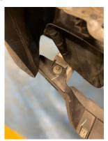
8. Remove two T25 Torx bolts from underneath the rad pack then an additional two T25 bolts from the top. Remove the end take covers from the sides of the radiator by pulling them.
