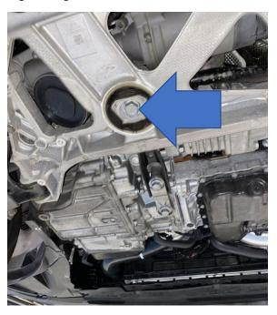
3. Insert your AIRTEC Motorsport billet insert and then reinstall the bolt. You may need to lever the engine towards the back of the car slightly to realign the bolt with the hole. Use a torque wrench to tighten the bolt to 130nm/96lb ft.
