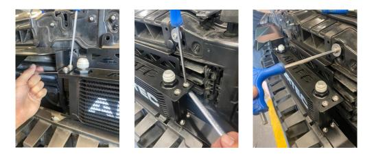
12. Reuse two of the plastic trim clips removed in Step 7 and install them into the bracket using their original locations.
