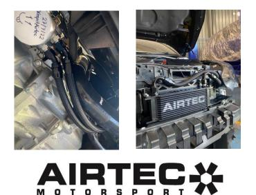
16. Install the line separators onto the lines as shown. The first is mounted before the headlight and the second by the bolt hole in the gearbox. Once happy that everything has been fitted correctly fully secure the oil lines by using an adjustable spanner.
