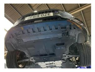
2. Now you can remove two T27 bolts from either side of the wheel arch liners.
