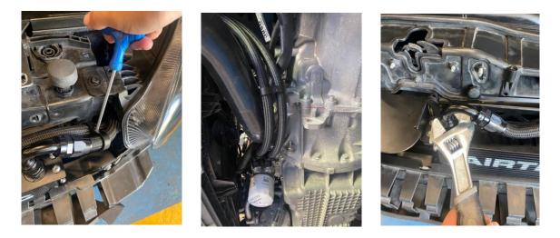
17. Finally, top up with 0.5 litres of oil and check the level and that all of the fittings are dry. Once the car is run up to full temperature, check the oil level again and top up as required.
