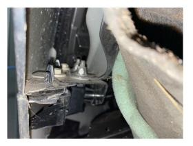
5. Release the bumper from the wing brackets by firmly but carefully pulling from the car.
