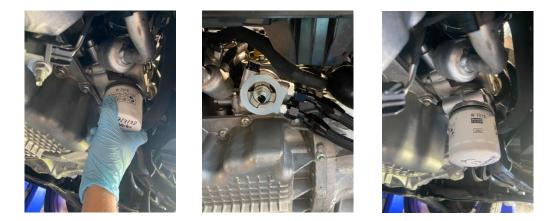
15. The oil lines can now be secured loosely by hand onto the oil modem and oil cooler, the shorter oil line will need to be mounted on the right side of the oil cooler. Make sure that they don't twist and have a smooth flow from the mounting points.
