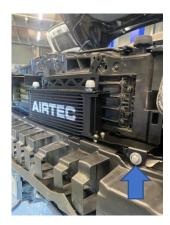
11. Now you can secure the oil cooler to the air guide by using two M6x16mm Button Head bolts with M6 Pan Washers and M6 Nyloc Nuts. Then use the remaining fixings to secure the other end of the oil cooler and then fit the supplied M6x16mm Socket Head bolt with M6 Mudguard Washer to secure the top bracket to the car.
