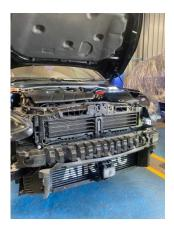
8. Remove the two 10mm bolts from the top of the crash bar. Now you can install the AIRTEC air guide in place by reusing two plastic trim clips and reusing the left-hand 10mm bolt.
