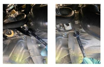
14. The oil filter will now need to be removed from the car, make sure that you have something in place to catch the excess oil. Then the oil modem can be secured in place using a 27mm socket making sure the oil line fixings are facing towards the side that the oil cooler is mounted. Now you can reinstall the oil filter onto the oil modem.
