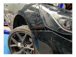
6. Now unclip the wiring harness from inside the driver's side arch liner and unclip two harness clips.
