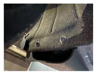
3. Remove six 10mm bolts along the top of the bumper, plus the two trim clips and two T27 Torx bolts.
