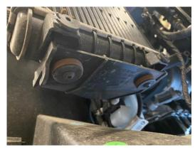
9. The AIRTEC Motorsport auxiliary radiator reuses the original mounting points, so slide it in position and then reattach the hoses onto the new radiator.
