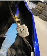
6. You will now have access to each of the auxiliary radiators. To remove the ducts, slide them across to allow the four locating pins to release.
