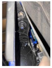
3. You may have an optional rubber trim attached to the bumper and wing. If so, remove this by gently pulling it away from the car. You can now firmly but carefully pull the bumper away from the wings on both sides of the vehicle.
