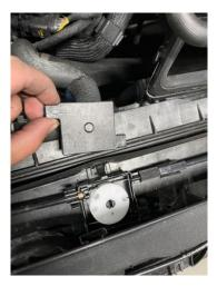
9. Remove the crash bar by unplugging the temperature sensor and horn. Then remove the eight 15mm bolts and four T25 bolts.
