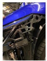
8. Unplug the sensor from the front of the rad pack directly underneath the bonnet latch, then remove the plastic cover from where the bonnet cables are attached and remove the left-hand side cable.
