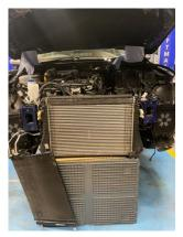
12. Remove the original intercooler by disconnecting the hoses.
