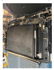
17. Finally, refit the crash bar, headlights, front bumper, arch liners and grille in reverse of Steps 1 to 10 and check everything is tight.
