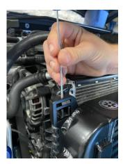
14. Refit the plastic tabs onto the new intercooler and reinstall the radiator cradle in reverse to Step 11. Then push the tabs back through the cradle and use the supplied self-tapper screws with washers to fully secure the intercooler in place, as shown.
