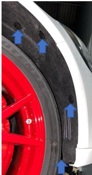
4. Remove air feed by pulling it back to release from the front bumper. There is a rubber bung by the battery that holds the rear. It can be removed and placed aside.
