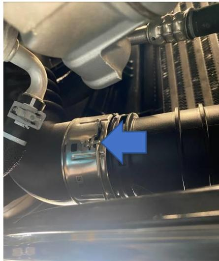
18. Remove the 7mm bolt holding the air-con pipe to the top of the original intercooler.
