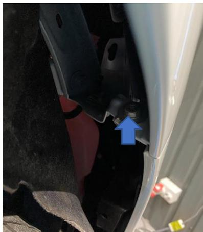
9. Remove three 10mm bolts on each headlight, disconnect the three plugs and remove the clip holding the cables to the headlight. Then remove and set aside.
