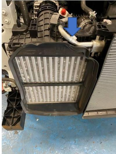
20. Remove the screw from the top left duct fitted and cut 12mm from the end of the thread to stop it from interfering with your new intercooler. Then refit.
