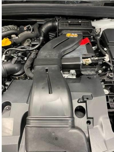
5. Undo the four T20 Torx bolts along the front panel.
