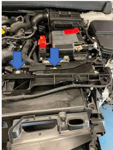
15. The front surround can now be removed by undoing the two 10mm bolts in each lower corner and the two 13mm bolts on the top one in each corner. Then lift the surround up over the pegs and remove from the car.
