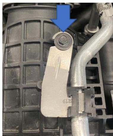
19. Using a flat-bladed screwdriver, unclip the intercooler and it can then be released from the radiator. Tilt the intercooler to the left and then lift to clear the air-con pipe, but do take care as you remove.
