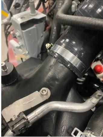
23. Reinstall the surround - you may need to undo these two 10mm bolts and position the bracket so it sits on the intercooler post. Once happy with the position, use the M6x16mm Socket Head bolt with 25mm washer to secure the post to the bracket.
