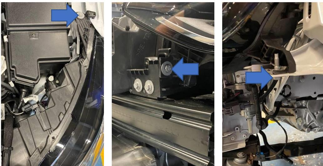
10. If your car has Active Cruise Control (ACC) then it will be located here. Unplug the wiring harness and undo the two bolts holding it to the plastic surround, which will then allow it to come off with the crash bar in the next step.
