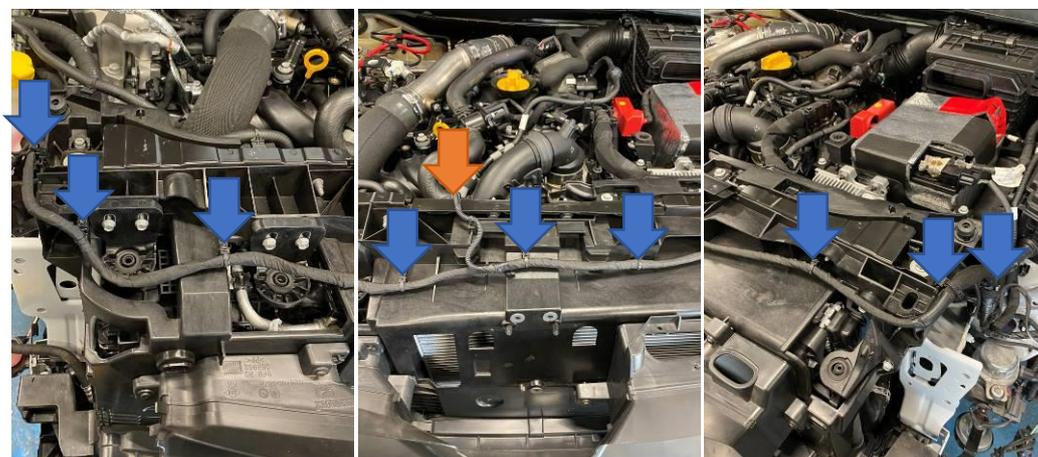
13. Release the bonnet latch by removing two 13mm bolts. Then move it to the side and out of the way without disconnecting the cable.
