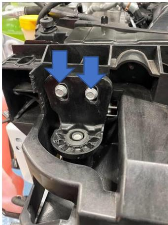
24. Finally, reinstall the parts removed in reverse of Steps 1 to 16.
