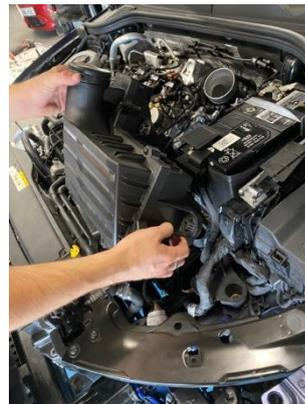
3. You will now need to replace the original hose with the new silicone hose provided. Remove the original by releasing the hose clamps at both ends. Then install the new one in place using the jubilee clips provided and tighten securely.
