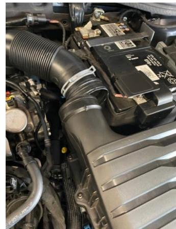
2. Remove the vacuum line from the air box by simply pulling it. Then lift the air box up and out of the engine bay, and place aside.
