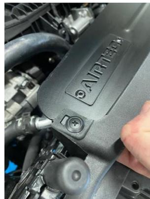
6. Fit the rubber mount onto the underside of the AIRTEC Motorsport air box, as shown. Then attach the air box onto the original mounting points and use three plastic push fittings to fix the air feed to the air box.
