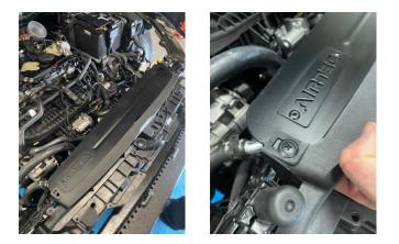
6. Fit the rubber mount onto the underside of the AIRTEC Motorsport air box, as shown. Then attach the air box onto the original mounting points and use three plastic push fittings to fix the air feed to the air box.
