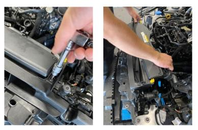
5. Now install the AIRTEC Motorsport air feed by aligning it with the original mounting points. Once in place, secure using the two plastic push fittings supplied, as shown.
