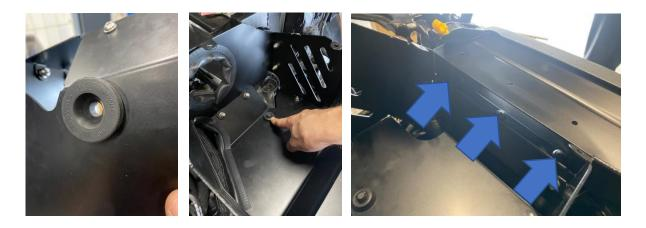
7. The intake pipework can now be placed into the air box and the filter installed onto the pipework using a hose clamp driver or flat-bladed screwdriver. The vacuum line can also be reconnected to the pipework as shown.
