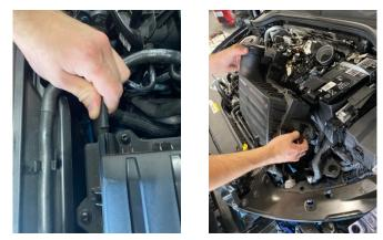
3. You will now need to replace the original hose with the new silicone hose provided. Remove the original by releasing the hose clamps at both ends. Then install the new one in place using the jubilee clips provided and tighten securely.
