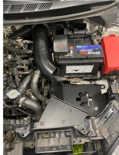
11. Finally, install the silicone reducer onto the AIRTEC Motorsport pipework using the supplied 100mm jubilee clip and then secure the air filter in place using the 120mm jubilee clip.
