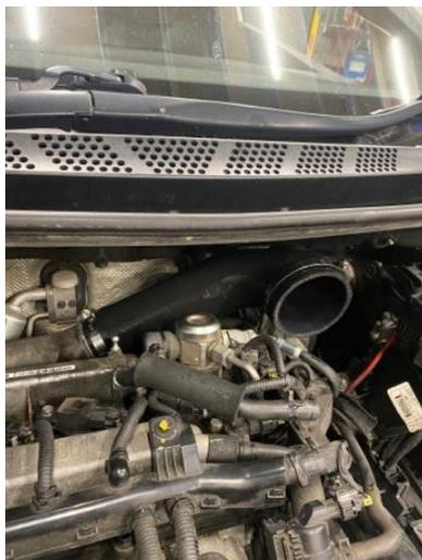
7. The AIRTEC Motorsport pipework can now be installed by sliding it into the silicone hose. Then reattach the two hoses removed in Step 2.
