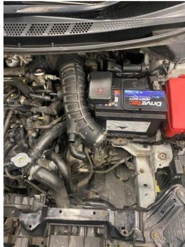
5. Remove the remaining pieces of pipework from the engine bay by loosening the clips using a 10mm socket or Phillips screwdriver.
