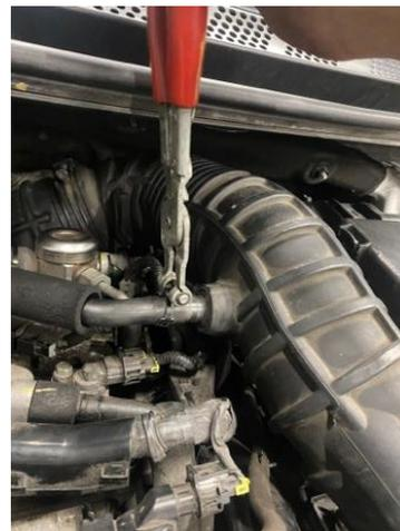
3. Loosen the jubilee clip from where the original pipework meets the air box, then remove the three 10mm bolts securing the air box in place.
