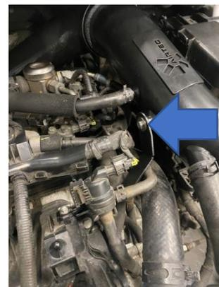
9. Install the heat shield by placing the spacer onto the threaded boss located on the chassis leg and then place the heat shield on top and attach using the supplied bolts.
