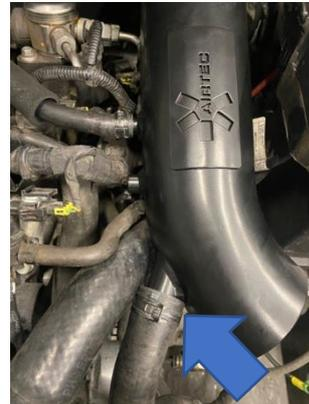
8. Remove the 10mm bolt shown in the picture below, then install the supplied bracket and refit the bolt. Then attach the bracket to the alloy pipework using the supplied M6x12mm Hex Head bolt with washer.
