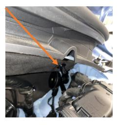
9. Fit the bracket onto this bulkhead thread using the M6 Nyloc nut and washer supplied. Once level and aligned, fully tighten the fixing.
