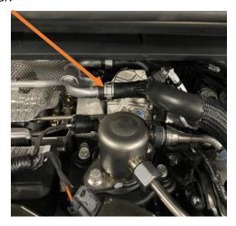
5. To remove the induction pipe, loosen the two hose clamps highlighted below using the pliers and then disconnect the hoses.
