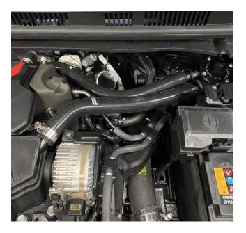
11. Re-install the induction pipe, foam cover for the fuel pump and the engine cover in reverse steps to removal. Check everything is tight and secure.
