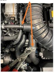
6. Undo the two 10mm hose clips highlighted and remove the pipe from the car.
