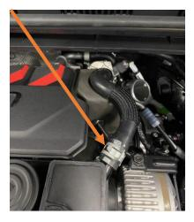
3. Remove engine cover from its rubber mounts by pulling at the bottom left corner and then pulling at the back. Once removed, take off the foam cover fitted over the fuel pump.
