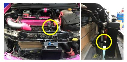
4. Fit 90 degree silicone hose from turbo to top outlet of turbo cooler Please note: 8mm ID end fits to turbo
