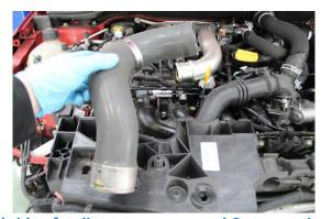
14. Lift left hand side of radiator support panel & remove intercooler
