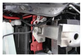
8. Unclip main right hand side air deflector cowling & slide upwards
