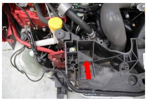
13. Remove top & bottom boost hoses, undo jubilee clips & unclip from front intercooler.
