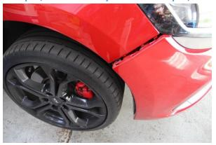
7. Remove crash bar x6 16mm bolts + un-clip wiring loom & 2x 10mm bolts securing right hand side air deflector.
