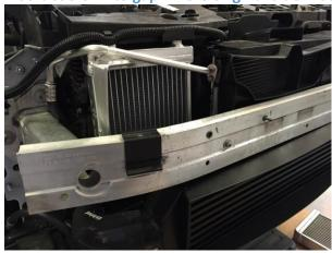
16. Drill through second plastic cradle and bolt M6 through onto M6 boss
