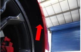
4. Remove x6 T20 screws from top of bumper.
