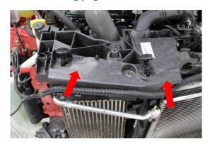
12. Remove 13mm bolt on top left of radiator support panel.
