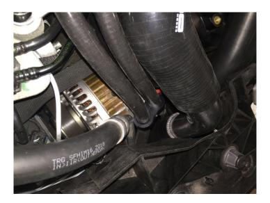
20. Attach second billet hose separator with attached aluminium bracket and bolt to engine mount by removing one 13mm bolt
