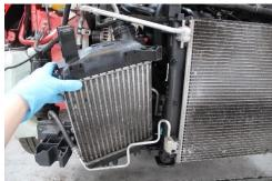
15. Insert cooler into gap where original side mount was located
