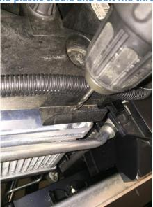
17. Drill self-taper screw into plastic behind light wiring loom cradle
