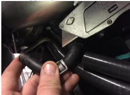
23. Insert billet connector and attach second silicon from top of turbo cooler.
