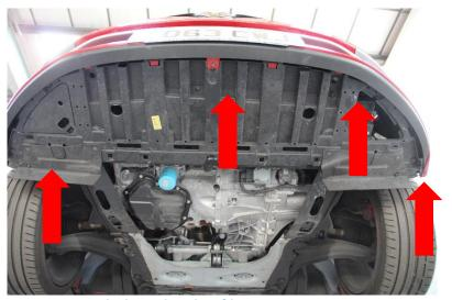
3. Remove 1x 10mm bolt each side of bumper.
