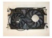
**3.** Fitting your Air-con radiator onto your Alloy radiator use's the x3 rubber grommets, these attach to 3 of the corners of the Air-con rad then carefully slide the rad across so that all 3 grommets are on your new rad
