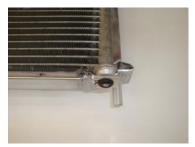
**4.** Then cable tie the 4<sup>th</sup> corner to secure, as shown below 'Do not remove Air-con radiator from car.
