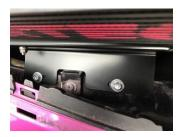
3. Fix oil lines to oil cooler. With 45 degree fitting closest to drivers wing. Secure oil line to fixing bracket with supplies P-clip
