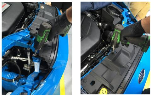
3. Undo bonnet release cable from release handle
