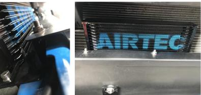
**11.** Run oil lines from oil filter housing between radiator cradle and onto oil cooler. Fixing to gearbox with supplied bracket and hose separator as pictured
