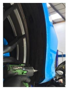
5. Remove plastic fixing clip holding bumper to arch
