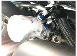
**10.** Bolt oil cooler into place onto original fixing tabs on front crash bar with supplied M6 x 16 hex head bolts
