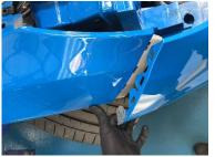
8. Remove bumper making sure to unplug loom on passenger side
