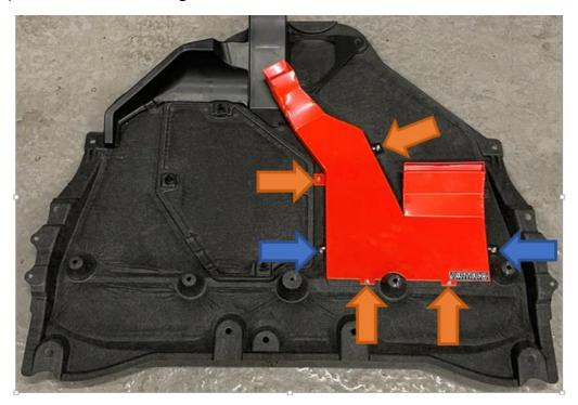
4. Once the holes are drilled, secure the cooling guide in place using the supplied Button Head Bolts with Nyloc Nuts, using washers each side. Tighten securely, check that the fitment is correct and then you can reinstall the undertray in reverse to the removal steps.
