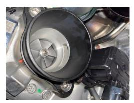
5. Finally secure the pipework using the supplied jubilee clips and tighten with a 7mm socket or flexi driver, now reinstall everything that has been removed in reverse of removal.
