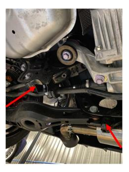
2. Now you can install the cooling guide by securing the front of the guide in place using the provided M6x20mm Socket head bolt with a washer, do not tighten fully as you will need some movement to align the rear of the guide.
