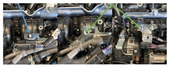
12. Unclip the pictured plug by pushing in on the blue button and pulling the plug backwards.
