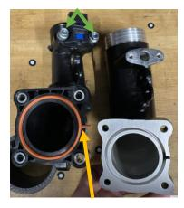
19. Reinstall your new Airtec motorsport elbow back onto the car by reusing the original bolts, making sure you sandwich the throttle body in between the elbow and the inlet manifold.
