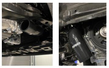
26. Install the new pipe and once happy with the position reuse the original bolts to install on to the car, tightening the left hand bolt first. Once installed and happy with the silicone positioning tighten the jubilee clips.
