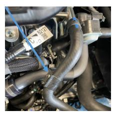
10. Undo the 3 x 10mm bolts holding the coolant hard pipe above the inlet manifold and move the hard pipe back so that it is out the way.
