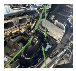
18. The Undo the 2 x 10mm bolts holding the MAP sensor to the elbow and swap it on to your new Airtec motorsport one reusing the original bolts, remove the gasket from your original one and place it into the groove on your new one.
