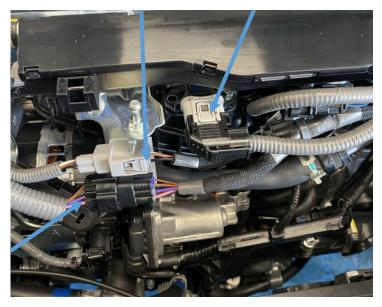
7. Undo the 10mm nut from the alternator and unclip the plug below. (This is a live cable and so please take appropriate precaution when undoing this and moving the cable out of the way, we recommend you disconnecting the battery which is located in the boot before this step.)
