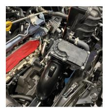
20. Reinstall the rest of the inlet manifold in the reverse of the above process. The wiring harness will clip back and bolt back in reusing the original bolt, the bracket can also be reinstalled using the original bolt. Once the inlet manifold is bolted back in go back and tighten the 12mm bolt that was loosened in step 14.
