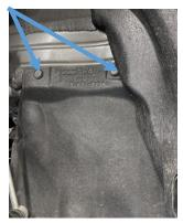
24. Undo the jubilee clips holding silicone hose to the intercooler and also the one holding the silicone to the turbo. (If you already have our intercooler installed the jubilee on the intercooler will be a 7mm however if it stock then it will be 10mm) Undo the 2 x 10mm bolts holding the pipe to the chassis and then remove the whole assembly from the car.
