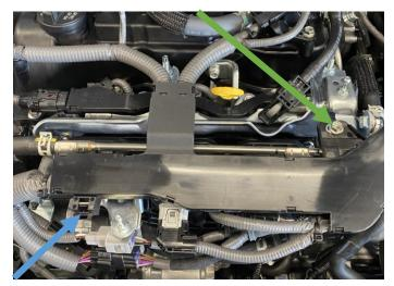
9. Unclip the coolant line from the breather line by removing it from the clip.
