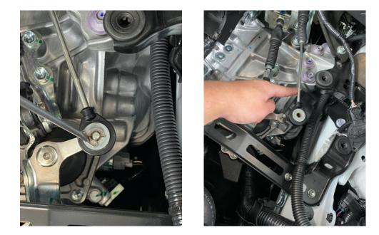
8. Install supplied washer onto the pin on the underside of the AIRTEC quick shifter.
