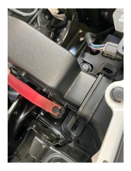
4. Unplug the vac line from the front of the airbox then unclip the line where secured on the air box.
