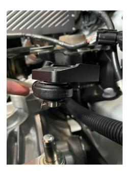
10. Install the top side of the short shifter on top of the stock pin, now align both parts of the short shifter and secure together using the supplied 4mm Allen key bolts
