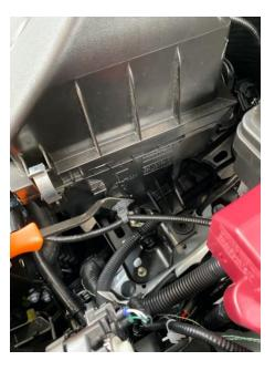
6. You can now remove the airbox by lifting from underneath.
