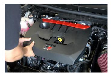
1. Start by removing the engine cover by lifting each corner and pulling away.
