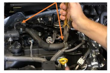
3. Install the lower part of the bracket to the front slam panel as pictured below, using the supplied M6 bolt and washer go through the existing hole in the underside of the slam panel.
