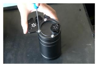
5. Mount the catch can into the engine bay using the x2 M8 bolts and washers supplied.
