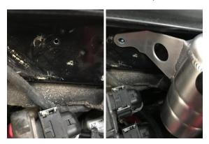
6. Secure breather tank to bulk head with supplied self-tapping bolt
