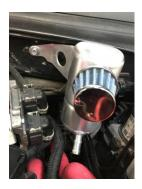
7. Attatch 14mm breather hose to OE breather outlet on gearbox and 10mm hose to barbed fitting.
