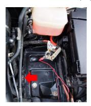
3. Remove battery tray by undoing 3x 13mm bolts as pictured
