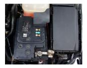
2. Remove battery by undoing 13mm bolt securing clamp. Location pictured below.
