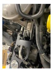
8. The washer bottle hose can now be installed onto the catch can mount and slide the provided fitting into the straight end of the hose as shown. Once fitted, you can push this end of the hose down into the washer bottle.
