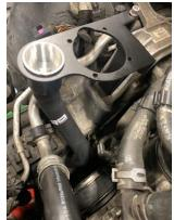
9. Install the catch can onto the bracket by using the supplied M5x8mm bolts then install the breather lines onto the catch can. Install the breather line from the silicone pipe down to the right-hand side of the catch can.
