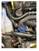
6. Remove the 10mm bolt securing the washer bottle in place, then lift the washer bottle out and remove the 13mm bolt from the engine mount.
