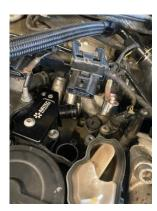
5. To create clearance and prevent any rubbing on the new breather hose, first you will need to use a hose clamp tool to release the clamp pictured and spin it around.
