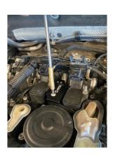
3. Remove the breather pipe from the intake pipe by applying pressure to both sides of the clip to release it. Once removed, install the longer 90-degree breather hose onto where the original one was removed. Push the metal clip down to ensure it's fixed in place correctly.
