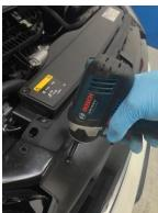
2. Undo 6x T30 Torx securing metal scuttle ends above headlights.
