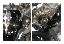
17. Remove water pump by undoing 5x T27 torx bolts and unclipping water feed pipes
