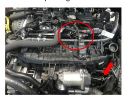
12. Remove cold side boost pipe from throttle body to intercooler
