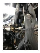
16. Remove plastic cover covering water pump belt 2x T27 bolts. Once removed, remove belt.
