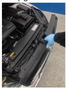
4. Undo 6x T20 Torx holding inner arch to bumper.
