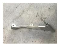
14. Remove manifold making sure to block inlet holes to avoid anything dropping in
