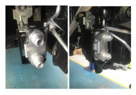
23. Fit oil lines to thermostat and oil cooler, at this point attatch oil cooler to crash bar, mark mounting holes and drill with 6.5mm drill bit, then bolt oil cooler into place with supplied bolts.— PLEASE SEE DIAGRAM AT END OF INSTRUCTIONS FOR OIL FLOW
