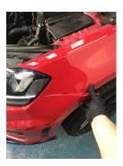
8. Remove bumper making sure to unclip multi plug and headlight washer pipe.
