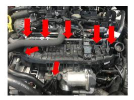
11. Unclip wiring harness from manifold
