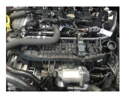
10. Undo 10x T27 torx sockets, undo 2x T27 securing water pipe
