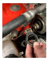
2. Now remove the 8mm nut securing the EVAP unit bracket to the engine bay. Once removed, there is access to remove the 18mm bolt from the side of the engine mount.
