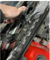
5. With the lower bracket removed, you will now have enough access to loosen the other 18mm engine mount bolt. Once removed, you can then slide the engine mount out.
