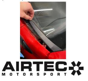
4. Remove the rubber weather seal by gently pulling it back and then remove both window wipers using a 15mm socket. The upper part of the scuttle panel can then be removed, revealing five 10mm bolts that will release the lower support bracket.
