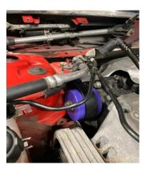
8. You can now start to fit the second bolt. The easiest way to locate the mount in place is to use a small pry bar or flat bladed screwdriver. Use these to align the holes and/or lever into place using the bolt hole and the inside of the mount's bushing. Once in line, tighten the bolts securely and reinstall everything in the reverse of removal.
