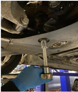
2. Now remove the second 21mm bolt going from the mount to the bracket secured to the engine.
