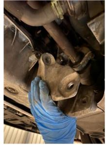
4. Now you can install your new AIRTEC Motorsport lower engine mount by sliding the mount into position and then reinstalling the 21mm bolt - **but do not fully tighten yet**.
