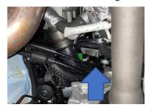
4. Remove the O-ring from the original connector and fit it into your new AIRTEC Motorsport connector. Then reinstall onto the vehicle reusing the clip.
